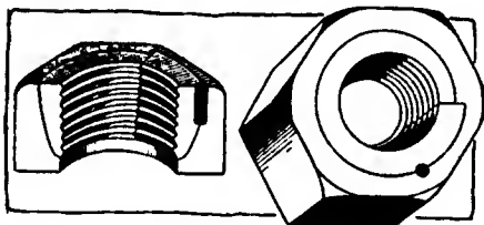
Fig. 3—Tite-Wad self-locking nut
